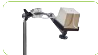
EMT (electromagnetic tracking) generator is positioned near the patient
